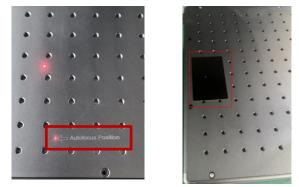
2. Press the autofocus button and wait a moment for the laser arm to move up and down to complete the autofocus.
