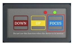
3. After focusing, move the object to the position indicated by the red light, then press the 'Start Engraving' button to begin marking
