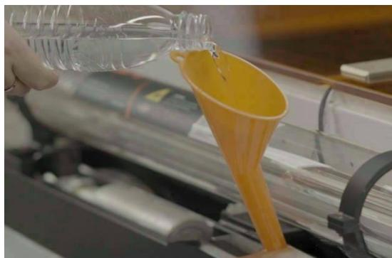
**Step 4:** Turn on the machine to activate the water pump. It will automatically circulate water through the pipe.
