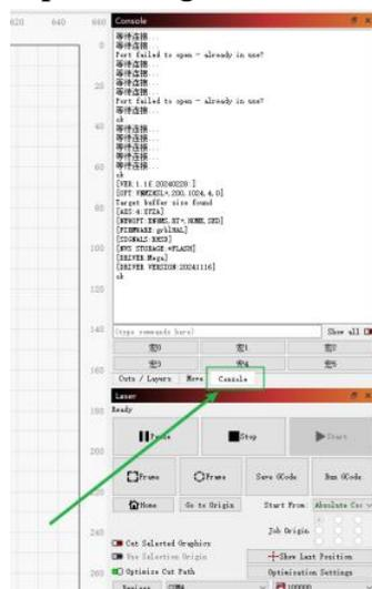
**Step 4:** Enter the following commands in sequence to set the optimal acceleration and deceleration parameters:
