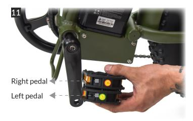
Install the pedals. No tools are necessary; you can easily secure them by hand.
