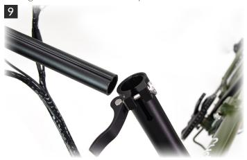
Insert the stem into its position while the headtube is folded.
