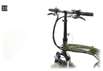
After placing the stem in position, lift the latch upward and push it to securely lock it in place.
