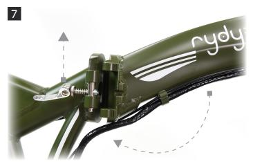
Lift the latch and unfold the bike completely while keeping the latch raised. Rotate the latch to the right and tighten the lever to securely lock the frame.
