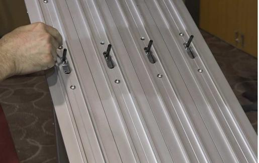
Attach gate to the bottom of the track. Bolts go through the two outside lanes.
