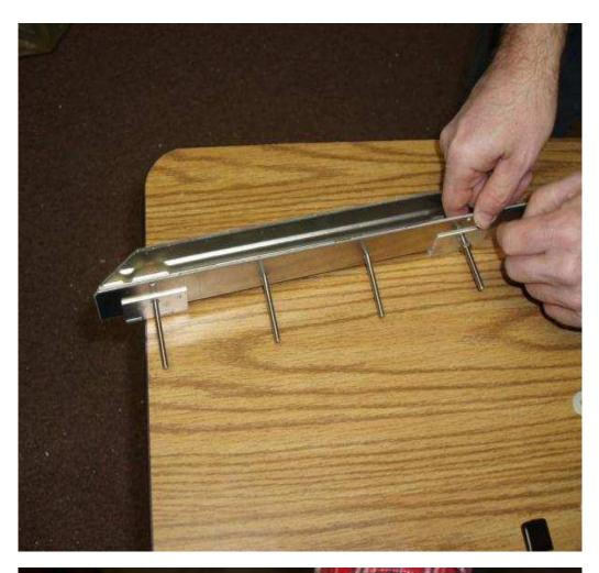
With the gate 'folded', attach the two springs to the small holes at either end.
