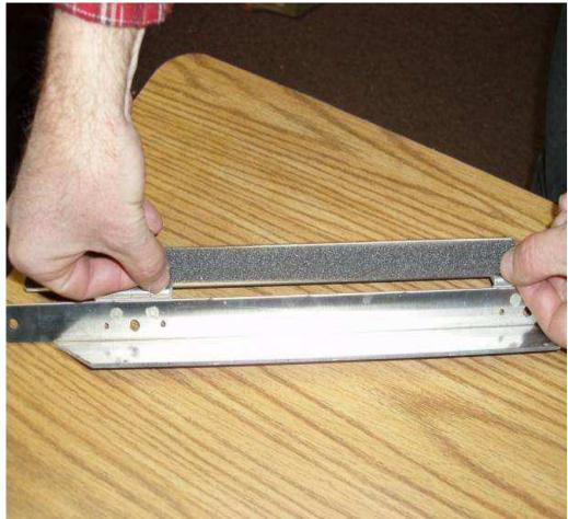
Attach the starting pegs. Feed the #10-32 x 2" screws from the bottom of the swinging gate and attach the nuts.
