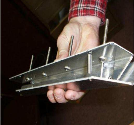
Next, place the 1/4-20 x 3/4" screw into the tab on the start gate.
