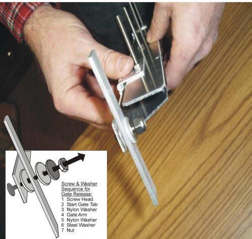
Press nylon screw into hole of the lever. Slip the black vinyl cover onto the other end of the lever. Slip the black vinyl sleeves over the starting pegs.
