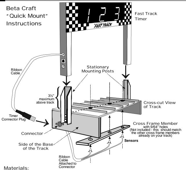
2 Stationary Mounting Posts, 1 Ribbon cable with sensors-attached to connector, & 6 Pan head sheet metal screws
