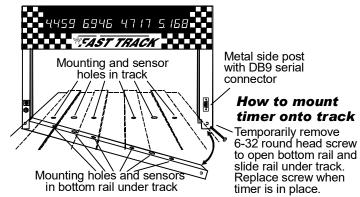
Once these holes are drilled, you are ready to mount the Fast Track finish line to your track. Remove the screw in the bottom corner of the finish line opposite the power jack. With this screw removed, the finish line can now hinge open. (If you remove the wrong screw, it can't be opened due to the wires running to the sensors). Remove and save the mounting screw.
