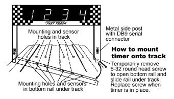
Once these holes are drilled, you are ready to mount the Fast Track finish line to your track. Remove the screw in the bottom corner of the finish line opposite the power jack. With this screw removed, the finish line can now hinge open. (If you remove the wrong screw, it can't be opened due to the wires running to the sensors). Remove and save the 2 mounting screws.
