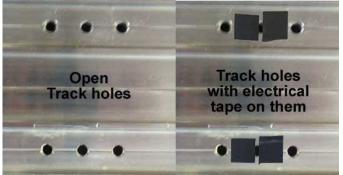
We have used J-B Weld, or J-B Kwik epoxy to fix holes that were too big. You can fill the big hole with the epoxy, then redrill them to a smaller size. The new hole is a flat gray color that works well.
