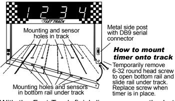
Once these holes are drilled, you are ready to mount the Fast Track finish line to your track. Remove the screw in the bottom corner of the finish line opposite the power jack. With this screw removed, the finish line can hinge open. (If you remove the wrong screw, it can't be opened due to the wires running to the sensors). Remove and save the 2 mounting screws.
