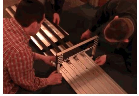
5. Test the Braking System alignment by running cars down the track.
