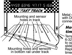
Metal side post with DB9 serial connector
