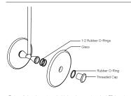
\*Ensure the rubber o-rings are installed in the correct position, 1 behind the glass, and 1 in-front on the glass. If the glass is not held firmly when the threaded cap is fully screwed in, install an extra o-ring.
