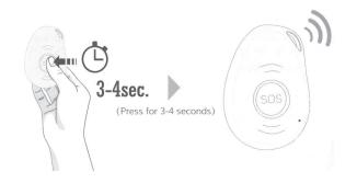
**Fall Detection:** When the device detects a fall it will automatically activate the SOS Alarm and connect you with an operator.
