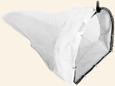
A D-frame fine-mesh dip net for collecting macroinvertebrates.
