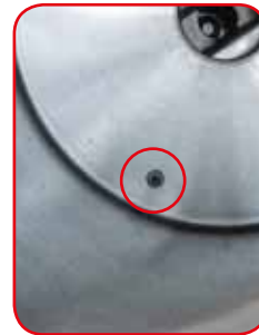
Probe in direct contact with the mix
