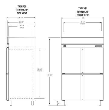
Cabinet designed for optimum performance in air-conditioned area at 70°F to 75°F ambient temperature and 50% to 55% relative humidity.
