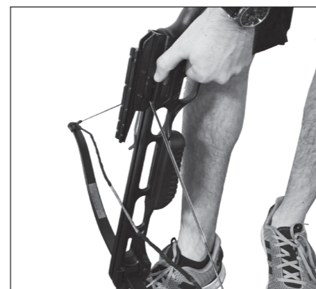
STEP 13: Cock Stringer Rope - Part 1 With foot firmly on the ground in stirrup for stability, slide the operating switch from the "Safety" to "Fire" position. Ensure there are no other persons near the bow, then pull the trigger. The bow will fire and is now strung.
