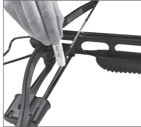
STEP 21: Lubrication Use provided lube wax and generously apply to the string and serving on the bow assembly and the flight track of the stock assembly.
