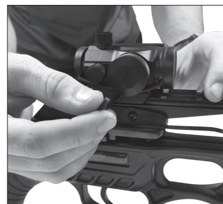
STEP 16: Attach Red Dot Sight - Part 2 Slide on the red dot sight, ensuring the metal latches grip the outside of the sight rail. Align and tighten with provided Allen wrench.
