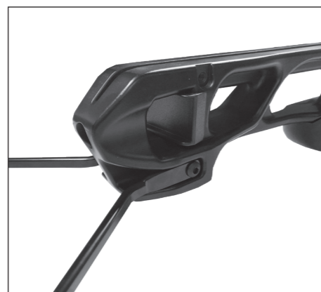
STEP 5: Insert Rear Pressure Pad Insert plastic pressure pad to the back of the limb slot as shown. The rear pressure pad should be positioned with the thinner flange on the top.
