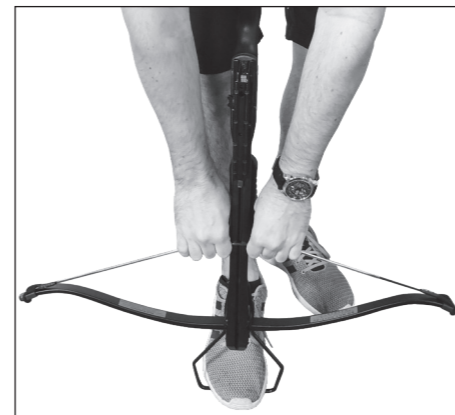
STEP 10: Cock Stringer Rope - Part 1 With foot firmly on the ground in stirrup for stability, pull the stringer upwards.
