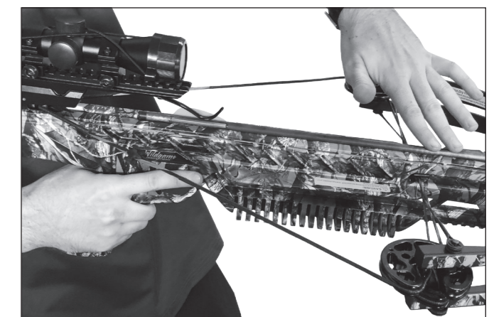
STEP 12: Load an Arrow Carefully place the arrow onto the flight track with the odd color fletch facing downwards into the flight track. Carefully push the arrow backwards until it makes contact with the string and is securely in place.
