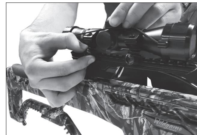
STEP 9: Attach the Scope Place scope onto picatinny rail as seen above, ensuring the metal latches grip the outside of the sight rail and the eye piece is a minimum three inches from the operator's eye when comfortably shouldered. Align and tighten the fixed screws.
