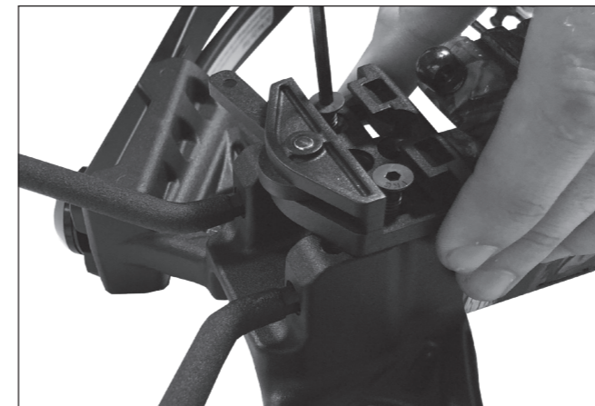
STEP 7: Quiver Assembly - Part 2 Screw in the quiver mount with two screws onto the bottom of the stock as shown. Tighten with provided allen wrench.
