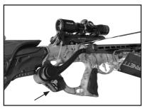
Step 6: Re-engage the CCD Latch by moving it from the "OFF" to the "ON" position once again.
