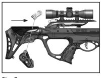
Step 3: Loop the RCD String Hooks around the back of the butt stock so the butt stock is now between the RCD String Hooks and the CCD Assembly, as shown above.
