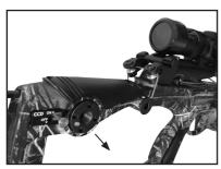
Step 8: Crank the CCD until the strings are taut and then remove the CCD handle. CAUTION: DO NOT OVER TIGHTEN. Over-tightening when cranking will cause damage to the CCD assembly.
