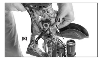
Step 4: Engage the CCD Catch Lever (A) to the 'ON' position (Closest position to the Butt Pad). Use one hand to hold and steady the crossbow and the other to rotate the crank handle (B).
