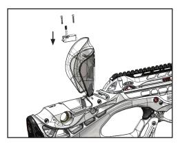
Step 2: Locate CCD catch assembly and the 2 x #4-40 x 3/4" socket screws.
