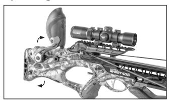
Step 5: Rotate handle until crossbow string is fully engaged into trigger mechanism. The safety of the crossbow will automatically engage. The tumbler latch of the trigger will now be holding the string.
