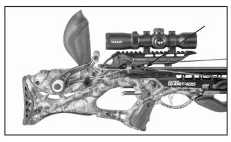
Step 6: Check to make sure the string is fully secured in the crossbow trigger mechanism and the safety is in the SAFE position prior to proceeding to step 7.
