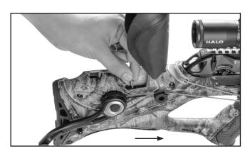
Step 7: Turn the handle to relieve the load on the lever, then move the CCD Catch Lever to the OFF position.
