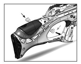
Step 8: Locate the two CCD anchors and the #10-24 x 1.25" socket screw from the assembly package. Make sure CCD string is properly in the CCD String Groove in the stock. Place one CCD anchor in each side of the stock as shown above with the flat portion of the anchor facing up. Fully tighten with the #10-24 x 1.25" socket screw.
