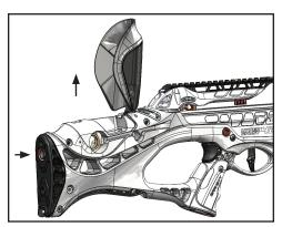
Step 1: Press the cheek rest latch button to open the cheek rest and reveal the CCD location.
