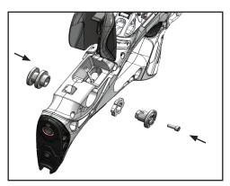
Step 4: Next, locate the CCD spool assembly with the string hooks. Remove the #10-24 x 1/2" socket screw from the spool assembly, allowing you to disassemble the two spools and gear. Place the right spool (with gear) into the right side of the stock, and the left spool (no gear) into the left side of the stock.
