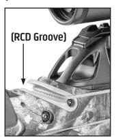
Step 7: Hook the string hooks onto the crossbow string, and bring the CCD string in between the hooks back behind the scope and into the RCD Groove (shown above).
