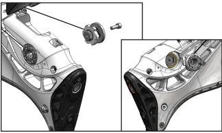
Step 5: Align the right spool's male insert portion correctly to the left spool's female socket as shown above. These always align so that the cords are also aligned ensuring these are installed in the correct position. Tighten the #10-24 x  $\frac{1}{2}$ " socket screw firm, using the CCD handle connected to the left spool to keep the spools from spinning while tightening the socket screw.
