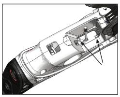
Step 3: Toggle the CCD catch lever to the front/left OFF position as shown above. Press the CCD Catch firmly down into the stock until snapped into place. Secure the CCD Catch Assembly using the #4-40 x 3/4" socket screws.
