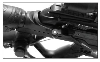
**Step 6:**Check to make sure the string is fully secured in the crossbow trigger mechanism prior to proceeding to STEP 7.
