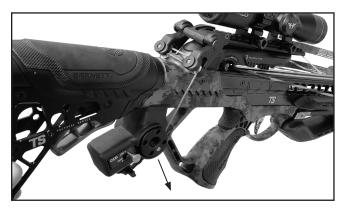
Step 10: Crank the CCD until the strings are taut and then remove the CCD handle. CAUTION: DO NOT OVER TIGHTEN. Over-tightening when cranking will cause damage to the CCD assembly.
