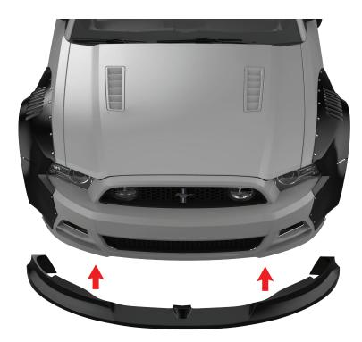
Remove your OEM front lip. Place SHIROKAI front lip onto the front bumper and tape it into place or do it with the help of an assistant. When drill holes into the bumper. Install cleco pins to secure the part and maintain proper alignment.
