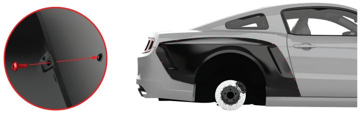
Carefully install the Flare onto the vehicle using the button head cap screws and washers. Start at the center and work outward. Do not fully tighten any of the fasteners until every one has been successfully started.
