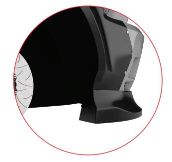
Make sure all parts are fitted well, chek all mountings, install your new bigger wheels and check inner fender volume with full load. Disassembly all body kit parts for painting
