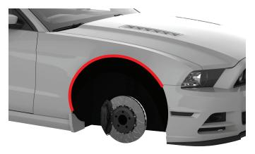
With the help of an assistant, hold the Flare up against the vehicle and trace the Flare and cut line with a permanent marker.
