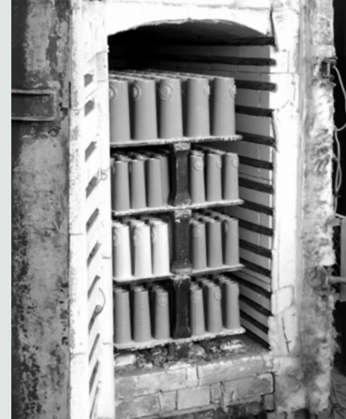
◆ Pipanellas in the kiln
