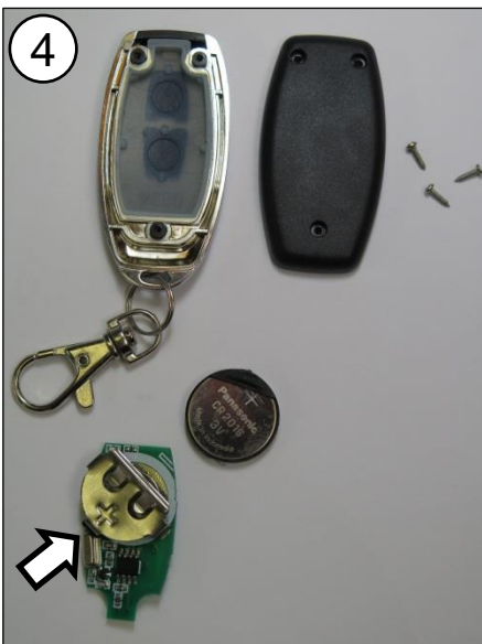
Gently slide out the battery pack which has a small plastic retaining hoop.
