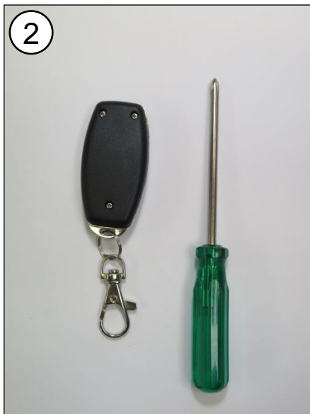
Remove rear cover by removing 3 off screws with a small Phillips head screw driver.
