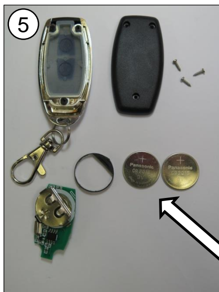
Remove and replace 2 off CR-2016 3V Lithium button cell batteries as shown and re-assemble.
