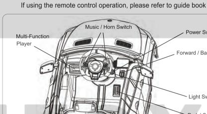
power switch, forward/backward switch, battery indicator, MP3 slot and volume adjuster are on the instrument platform, charging hole is on the front of the seat.
