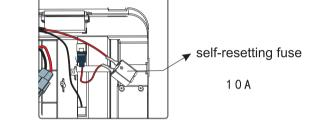
Cause: battery connector or wires are loose Make sure the battery connectors are firmly plugged into each other.
