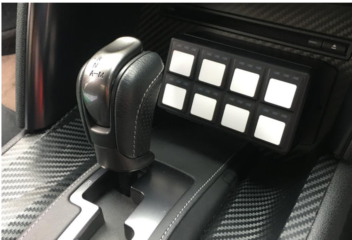
Figure 1.0 Example of an Emtron 8 Button CAN Keypad Fitment to a Nissan GT-R R35
