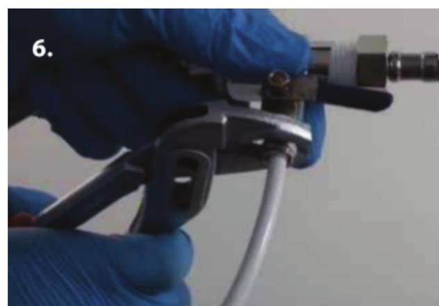
Push the tubing onto the stem of the ball valve. Ensure it has been pushed all the way over the little ridge.
