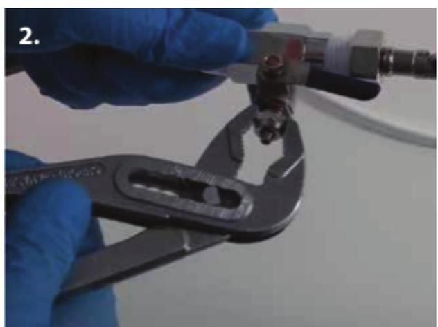
To connect the ball valve to the tubing for the water filter, start by removing the nut on the blue ball valve. Then place the nut over the tubing.
