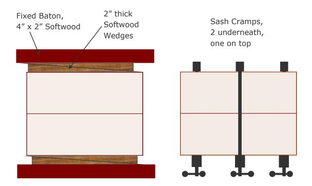
Next, either with sash cramps or with wedges, dry clamp the pair of boards together, planed faces mating. If your clamping method holds OK, unclamp, apply Titebond glue to both planed edges and re-clamp. Put a sheet of newspaper under the boards so you don't glue them to the bench!
