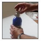
5. Reload with dry compressed air between 4 and 8 bars (test to see the best pressure for the product being sprayed)
