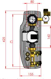
(\*) Distance of threaded connections: 22 mm compression end: 405 mm 3/4"M and 1"M: 385 mm
