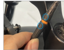
6. Link the light wires, and note that the arrow symbols of the terminals need to correspond to each other
