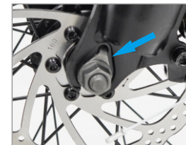
9. If it is necessary to snap the snap ring shown in the figure into the fork slot
