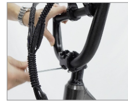
3. Torque the four screws of the carabiner
