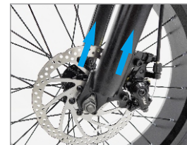
8. Insert the forks into the screw gap in the bearing
