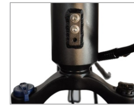
10. There are 3 holes in total, please select the top 2 holes for installation, as shown in the figure
