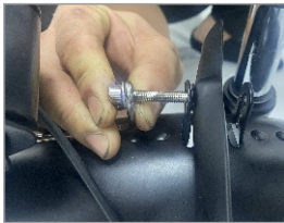
4. Put the screw into the lamp's mounting bracket, install it on the fender mounting bracket
