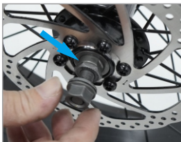
7. As shown in the figure, tighten the nuts marked at both ends of the central shaft
