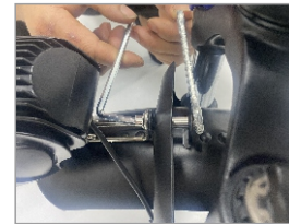
5. As shown in the picture, attach the remaining attachments with the screws to the fender mounting brackets and tighten the screws
