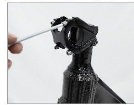
2. First remove the mounting clips, then install the U-shaped handlebars
