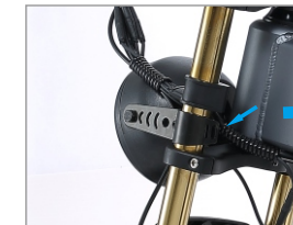
9. Insert the No. 1 fixing piece into the slot of the No. 2 fixing piece
