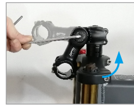
2. Adjust the position of the riser.
