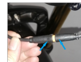
12. Link the light line, pay attention to the arrow corresponding to the direction of the arrow at the other end
