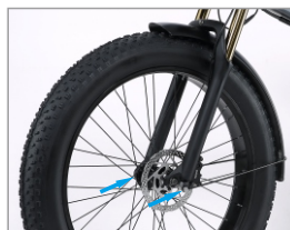
7. Install the fenders and tighten the screws
