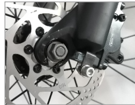
6. Tighten the left and right nuts as shown
