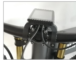
3. Install handlebar riser
