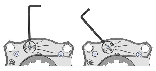
Now the regulation system is released. Remove the hex key and insert it in the socket of the regulation axis, on the central axis of the BRN.
