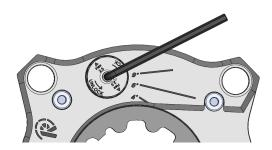
Slightly screw clockwise and the system reaches the  $9^{\circ}$ , the  $6^{\circ}$  and the last  $4^{\circ}$  position The lasered graphic shows the order and the reference distance between regulations.
