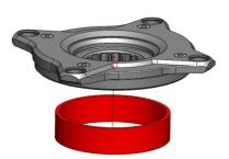
Unscrew all four m4x8 mm bolts using a 2.5 mm hex wrench.
