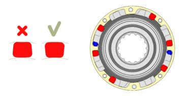
Close OCHAIN · E referring to lasered alignment marks "▼"
