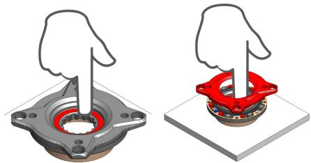
Replace all six elastomers with new ones, placing them as shown.
