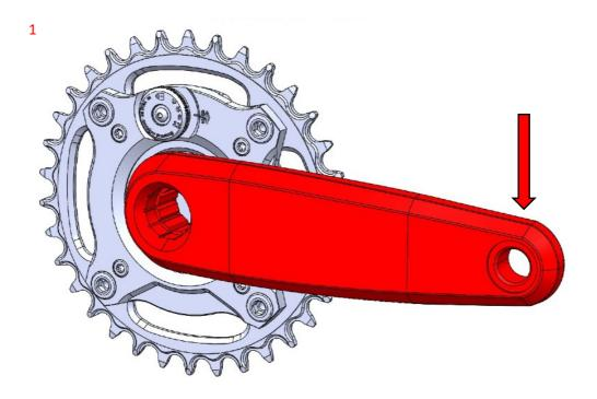
1. Push and hold the crank in pedaling direction in order to engage the ochain
