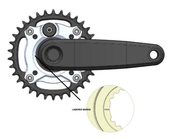
Fix the Ochain to the crank, with the lockring or the screws, referring to the manufacturer's manual for the procedure and the correct tightening torque.
