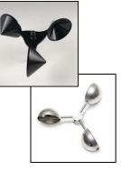
**Rotors: D2** (above), **D3** (top right), **metal**. D3 rotor introduced in February, 2020 The anemometer on the left has a "WS2" body
