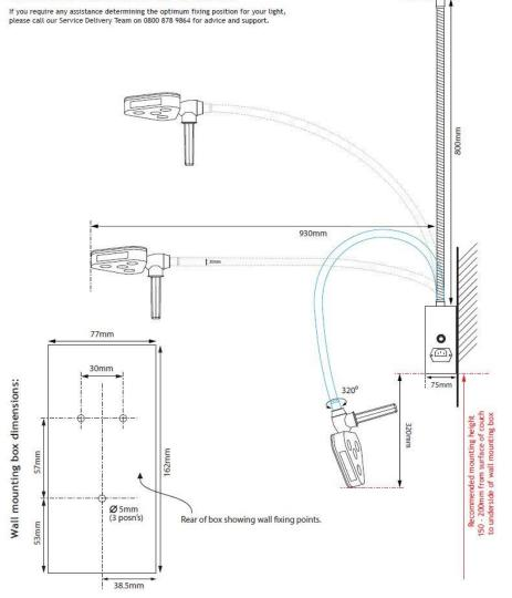
\*All dimensions shown in red are based on a suggested mounting height (see underside of wall mounting box). For specific applications and environments, the mounting bracket should be installed at a height so that, when fitted, the lighthead is as near to the required position as possible. Actual location should be dependent on intended use and desired reach. Common sense should always prevail.
