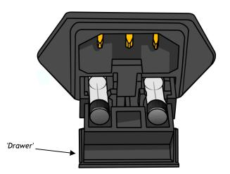
Unplug and remove IEC cable. Using a flat-bladed screwdriver, or similar, pull forward the 'drawer' containing the fuses. Hinge down the front of the holder. Lift the fuses by pushing them through the holes below.
