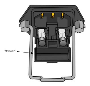
Unplug and remove IEC cable. Using a flat-bladed screwdriver, or similar, pull forward the 'drawer' containing the fuses. Hinge down the front of the holder. Lift the fuses by pushing them through the holes below.
