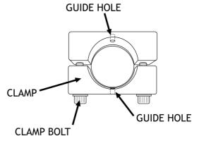
Tighten both clamp screws fully and evenly until the tube is firmly clamped.
