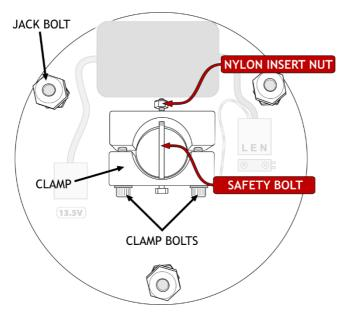
Fix the plate to the ceiling with bolts, screws or studs and nuts through the centre of each jack bolt. Do not fully tighten the fasteners at this point.
