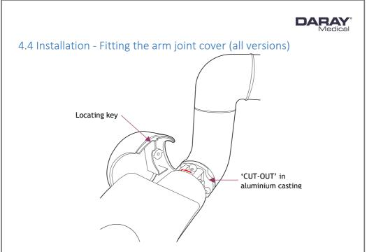
1. Covers are marked 'L' and 'R' on their inside faces as viewed from the end of arm. Engage the slider, with its 'T' mark uppermost, into the groove inside the cover.
