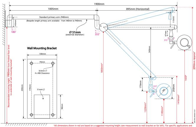
\*All dimensions shown in red are based on a suggested mounting height (see measurement to wall bracket on far left). For specific applications and environments, the mounting bracket should be installed at a height so that, when fitted, the lighthead is as near to the required position as possible. Actual location should be dependent on intended use and desired reach. Common sense should always prevail.
