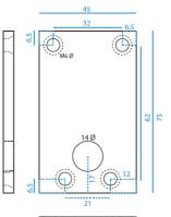
Backing plate dimensions and fixing points
