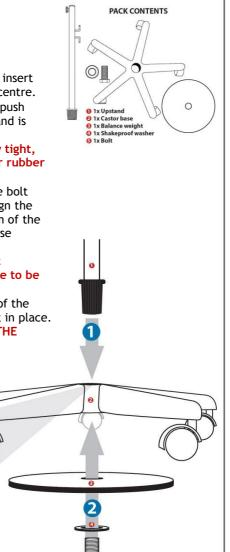
WARNING: If the upstand is not fully inserted into the castor base, it may become unstable whilst in operation
