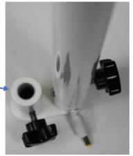
With the downtube directed it should be loosely fitted between the two metal clasps and then holes should be marked on the tube for where the safety bolt will go through; then remove the downtube and secure for drilling. A 7mm hole should be drilled through the downtube on both sides to allow the bolt to pass through.
