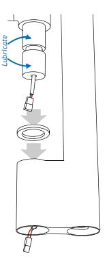
Then sit the connection inside one of the supplied bungs and insert the bung into the bottom of the downtube.
