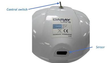
These controls can also be used to alter the lights variable intensity; push and hold the switch, or hold your hand in front of the sensor, to change the light intensity up or down.
