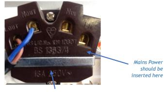
Fuse Holder around the front - 3 Amp Fuse - D15998
