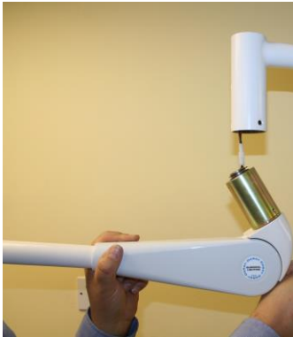
Fig.7 Making the electrical connection between the Rotation arm and the Suspension arm.
