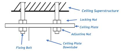
Depending on the choice of attachment method, fitting your ceiling plate will require bolts to be inserted into the ceiling superstructure. It is highly advisable that the plate being fixed to the ceiling, is secured with a minimum of 4 bolting points to ensure a complete and sturdy fit.
