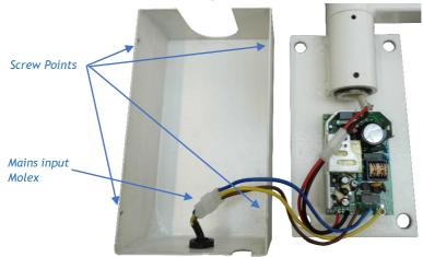
Supply power to the mains connection and power the light on using the button located on the lighthead. Check that all LED's illuminate.
