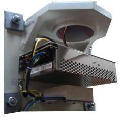
The SL400 Series lights should be connected to the mains supply via the transformer (pictured above). The cable used to power the light should be of a 1.5mm twin and earth type. Daray recommends that the power supply uses an earthed switched fused spur, protected with a 3 amp fuse.
