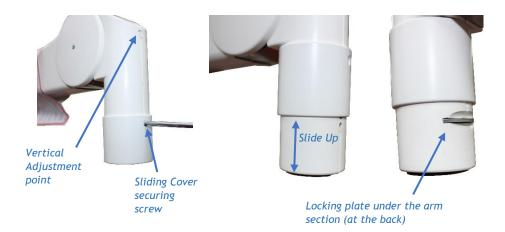
The standard system follows the same structure as the previous arm connection. No wiring is required for the inside of the arm sections, the connections are made using a powered spigot plug system. Grease the lower section of the spigot (not the plug) and slide the lighthead arm's spigot up into the rotation arm joint then re-insert the locking plate, slide the cover back down then re-secure it in place with the original screw.
