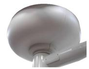
After installing the ceiling mount cover, we need to utilise the shroud left on the arm system in section 3.3.2 (page 18). Thread the shroud over the vertical ceiling boss, and over the ceiling cover, curved lip side first. This should sit snug against the top of the ceiling cover, hiding any gap between that and the ceiling.
