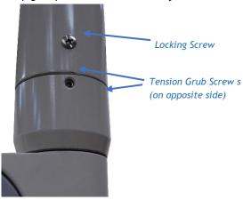
The lighthead is attached to a third arm system which incorporates the lights control panel. This arm also uses a plug system and can be connected straight to the suspension arm; remove the locking screw, ensure that the washer ring is placed on the spigot, grease the spigot and plug the arm in. Secure the arm with the locking screw and your lighthead is now attached.
