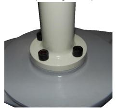
With the first section secured, you will need to attach the second section of the vertical tubing. You will need to unscrew the locking screw from the tubing section and ensure the tube is clear. Make sure the washer ring is in place on the first section of the vertical tubing and connect the wires from the upper section to the wires coming through the lower tube section. Once attached you will need to insert the two securing bolts shown.
