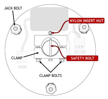
Fix the plate to the ceiling with bolts, screws or studs and nuts through the centre of each jack bolt. Do not fully tighten the fasteners at this point.
