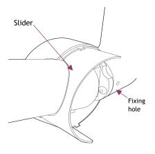
Align holes in cover and painted elbow. 'Nip up' the screw to secure. DO NOT OVERTIGHTEN
