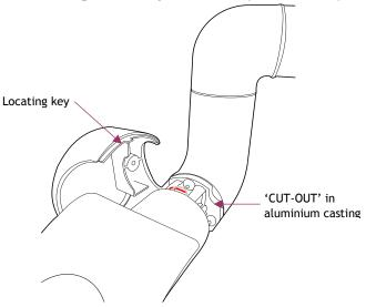
1. Covers are marked 'L' and 'R' on their inside faces as viewed from the end of arm. Engage the slider, with its 'T' mark uppermost, into the groove inside the cover.
