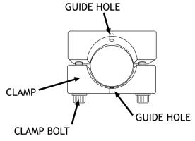
Tighten both clamp screws fully and evenly until the tube is firmly clamped.
