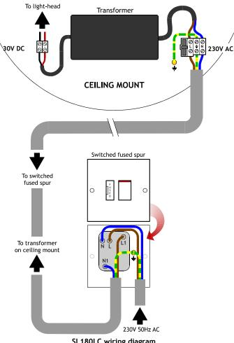
SL180LC wiring diagram
