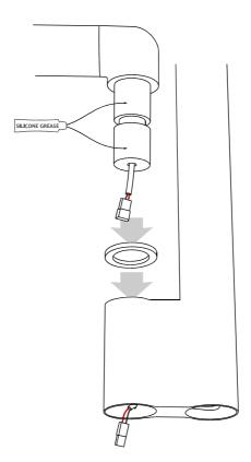
Join the connector from the primary arm to the connector from the down-tube.
