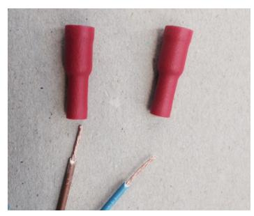
Crimp the Bullet connectors to the wires coming through the centre of the adaptor
