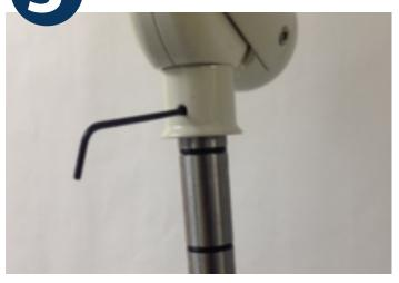
Loosen the grub screw and remove the bare spigot.
