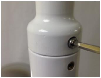
Insert the new head into the adaptor and secure using the grub screw supplied.
