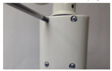
Remove screw which holds the C clamps together and then remove clamps to expose the contact panel.
