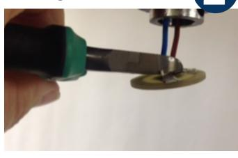
Cut the wires holding the contact panel, leaving the two wires showing.
