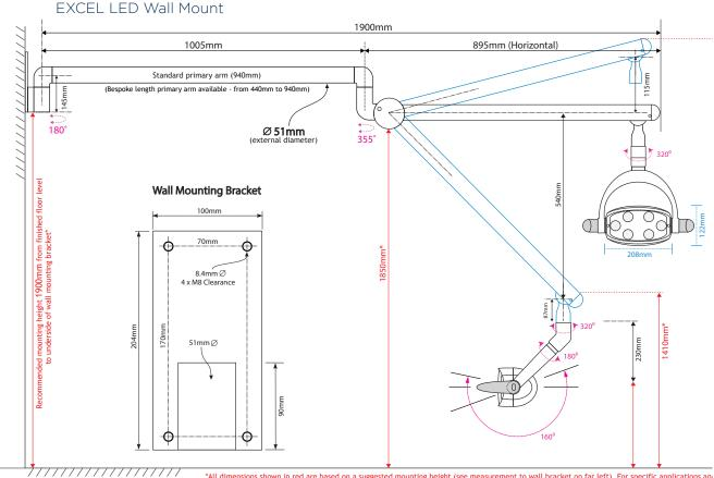
\*All dimensions shown in red are based on a suggested mounting height (see measurement to wall bracket on far left). For specific applications am environments, the mounting bracket should be installed at a height so that, when fitted, the lighthead is as near to the required position as possib Actual location should be dependent on intended use and desired reach. Common sense should always prevail.
