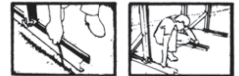
16. Repeat the procedure of step 13, 14 and 15 until all the pool frame construction assembly for your size pool is accounted for. At this stage temporarily install connectors to aid in finding alignment and levels.
